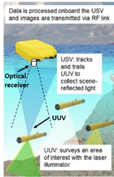
Figure 9. NIX capturing reflection from bistatic laser imager
