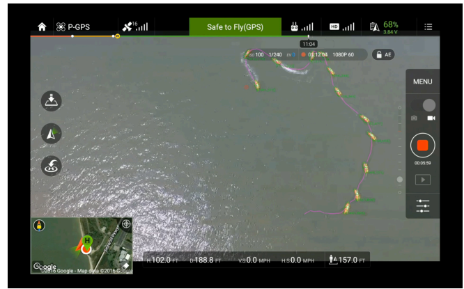
Fig. 2. EMILY visual navigation in Galveston Bay, Texas under strong wind (17km/h) and current
