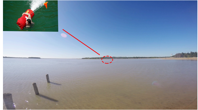
Fig. 1. Actual problem encountered by marine mass casualty rescuers: view point from USV operator. The USV and victim are not discernible from the view point at limited altitude on shore. Objects may actually be far apart, especially in perpendicular direction to shore, even though they appear to be very close due to perspective effect.
