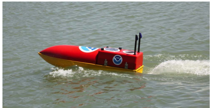
Figure 3. The EMILY Hurricane Tracker developed for NOAA as a platform to enter and gather persistent environmental data from within a hurricane.
